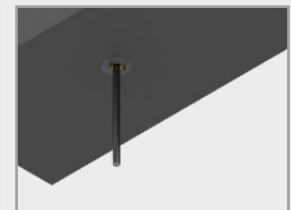
Confirm Engagement (Pull down on rod to confirm engagement)
